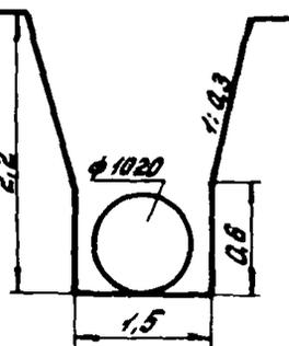
$V=4,1\text{ м}^3 \text{ на } 1\text{ м.}$
