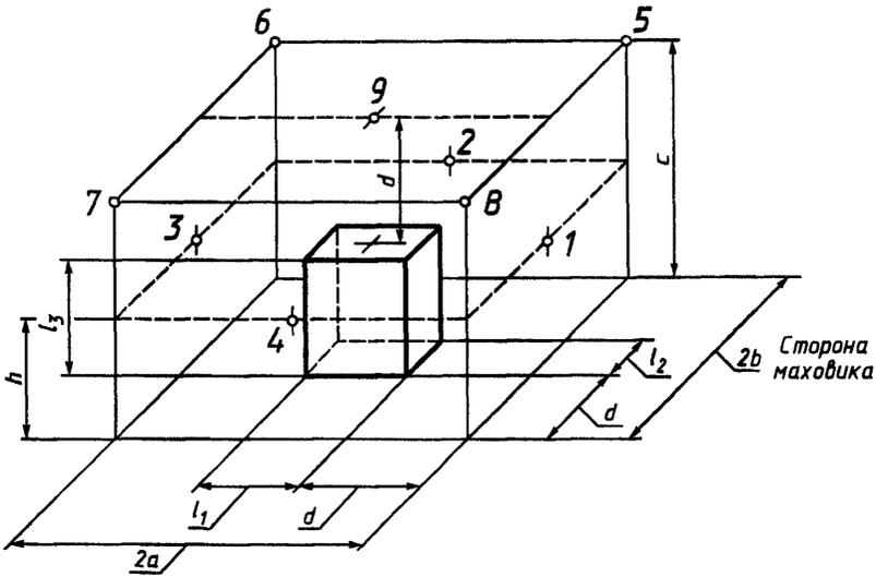
$$a = \frac{l_1}{2} + d; \quad b = \frac{l_2}{2} + d; \quad c = l_3 + d; \quad h = \frac{c}{2}.$$
