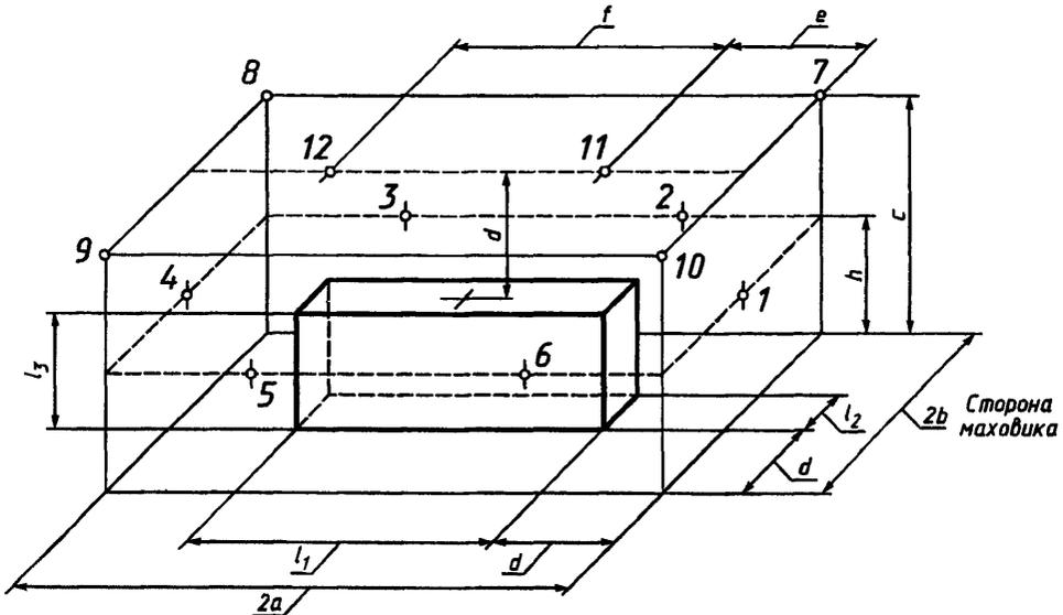
$$a = \frac{l_1}{2} + d; \quad b = \frac{l_2}{2} + d; \quad c = l_3 + d; \quad h = \frac{c}{2}; \quad e = \frac{a}{2}; \quad f = 2e = a.$$
