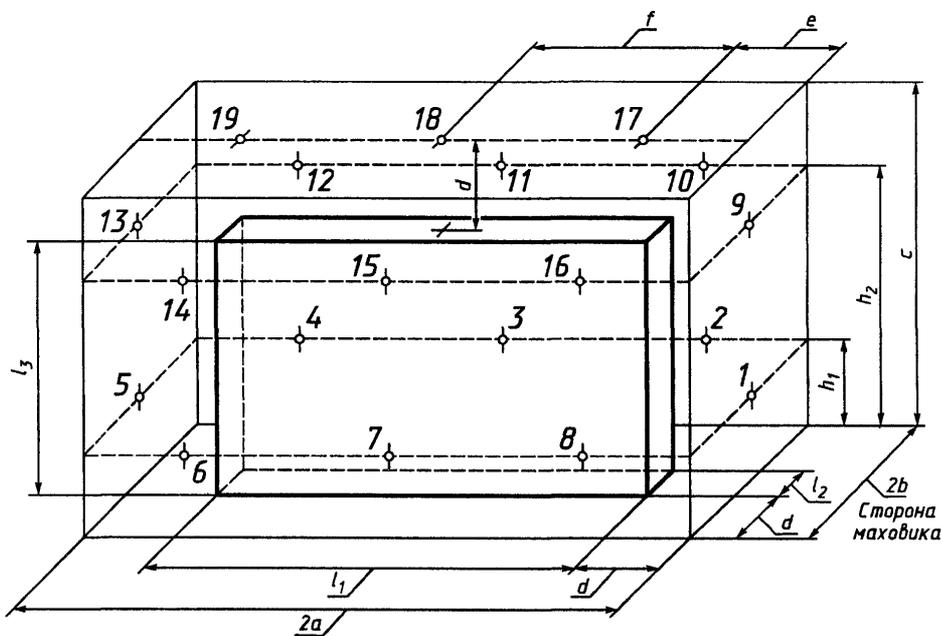
$$a = \frac{l_1}{2} + d; \quad b = \frac{l_2}{2} + d; \quad c = l_3 + d; \quad h_1 = \frac{c}{4}; \quad h_2 = \frac{3}{4}c; \quad e = \frac{a}{3}; \quad f = 2e.$$
