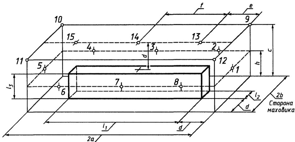
$$a = \frac{l_1}{2} + d; \quad b = \frac{l_2}{2} + d; \quad c = l_3 + d; \quad h = \frac{c}{2}; \quad e = \frac{a}{3}; \quad f = 2e$$
